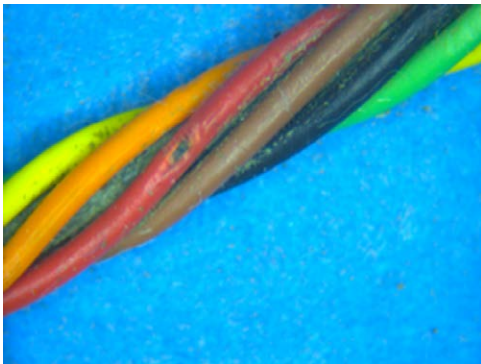
Figure 4. Damage to the percutaneous lead with insulation abrasion exposing inner wire strands to the silver-plated copper braided shield.
