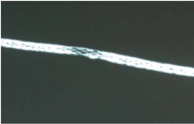
Figure 3. Radiograph image of breakdown of silver-plated copper braided shield.
